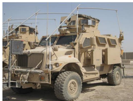
Mine Resistant Ambush Protected vehicle with Overhead Wire Mitigation Kits produced at Blue Grass Army Depot
