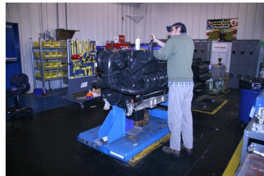
Overhauling vehicle engines at Red River Army Depot. Overhauled engines are returned to Supply Management inventory for sale to Army tactical units.
